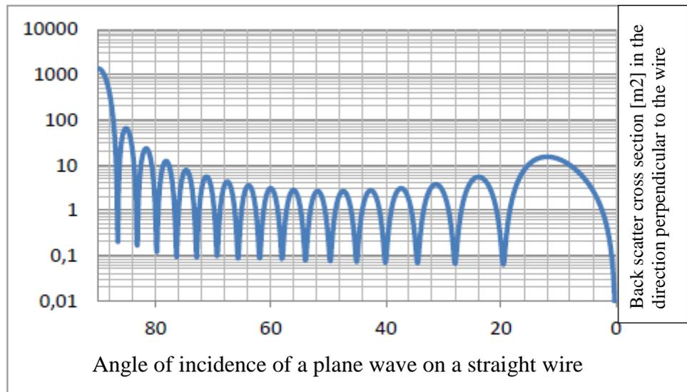
Figure E1: Back scatter cross section [m2] for the reflection direction perpendicular to the wire, for different angles of incidence of a plane wave with the thread @ 50 MHz, wire length 100 m, diameter 0.02 m, in 'free space'.
