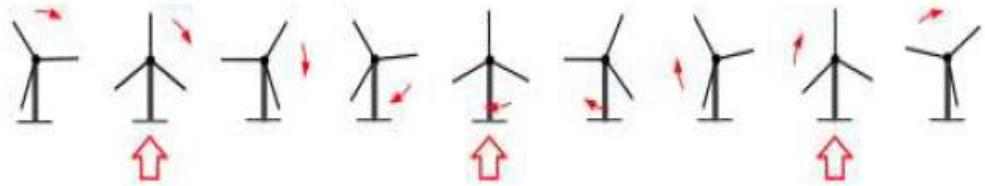
*The reflectivity of the wind turbine is dependent on the position of the rotor blades. The here drawn position of the rotor blades in which reflection occurs is only an example. It also appears that another (recurring) rotor position maximum reflection.*
