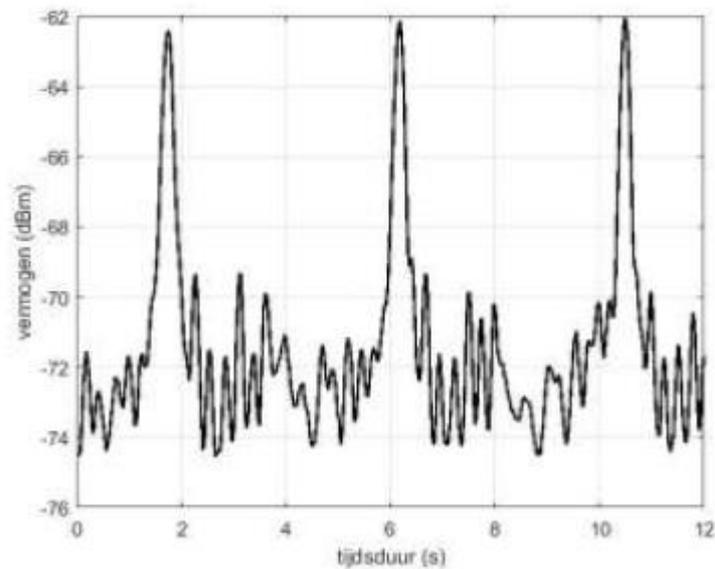
A detail of one of the reflectance measurements on a wind turbine, such as described in [15]. The regular reflection can clearly be seen. The repetition frequency of the reflection is dependent on the number of rotor blades and their rotation speed. The reflection is in each case of short duration and occurs at a very specific position of the rotor blades.
