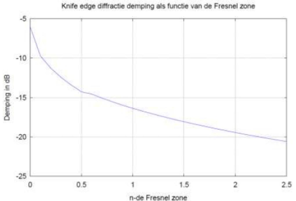
**Figure 8:** Knife edge diffraction as a function of the Fresnel zone [18]
