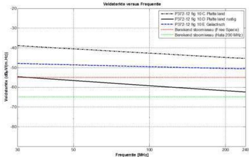
**Figure 4:** Electric field strength in dBµV / (m.Hz) as a result of one wind turbine at a distance of 5 km which complies with Class A EN55011 limits, [3], corresponding to a source strength of  $2.8 \cdot 10^{-12} \text{ W / Hz}$ . Calculations are performed with the 'free space' model and the 'Modified Hata model [14].
