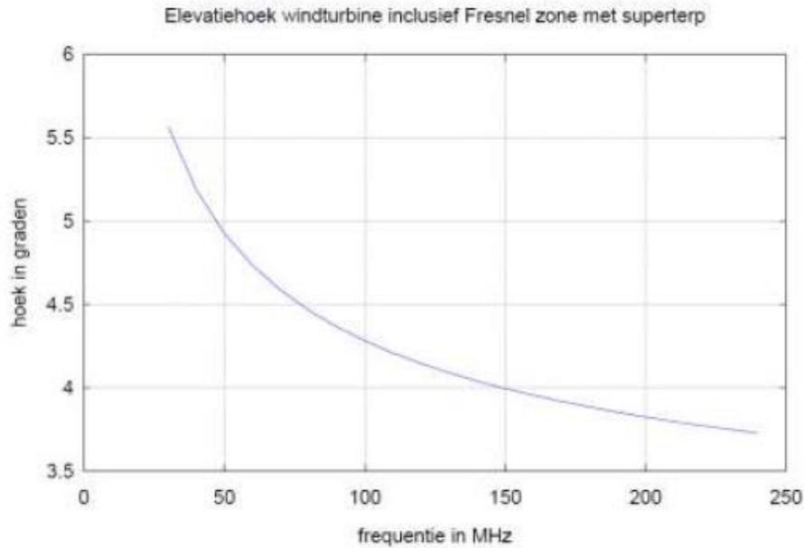
**Figure 9:** Observation angle (relative to the ground plane) such that no blocking and deflecting effects are to be expected, this as a function of the frequency.
