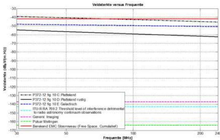
**Figure 10:** Overview of the level of interference as a result of the EMC emission of wind turbines (red line) and the different critical levels for performing radio astronomy measurements [22].
