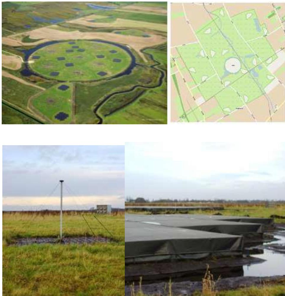
**Figure 1:** Upper left: LOFAR Super mound; top right: the LOFAR core (core), the circle indicates the super mound again surrounded by a number of stations. Lower left: antenna for the "low band (30-80 MHz) and below right: the 'High' band (120-250 MHz). Source: LOFAR website [11].
