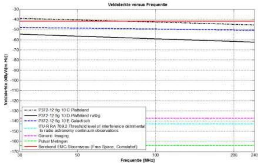
**Figure 5:** Electric field strength in dBµV / (m.Hz) as a result of all wind turbines together, each of which meet Class A EN55011 limits, [3], corresponding to a source strength of  $2.8 \cdot 10^{-12}$  W / Hz. Calculations here are performed only with the 'free space' model.
